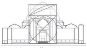
Fig. 10. Probable proportions of the original entrance portal compared to the restored portal. Source: Ansari & Nejad Ebrahimi, 2010, 41.
