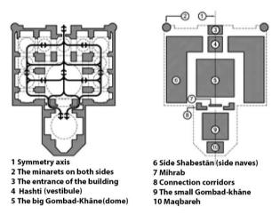
Fig. 3. The connection between the spaces of the Goy-Masjid, source: Kabirsaber, Mazaherian & Peyrovi, 2013, 11.
